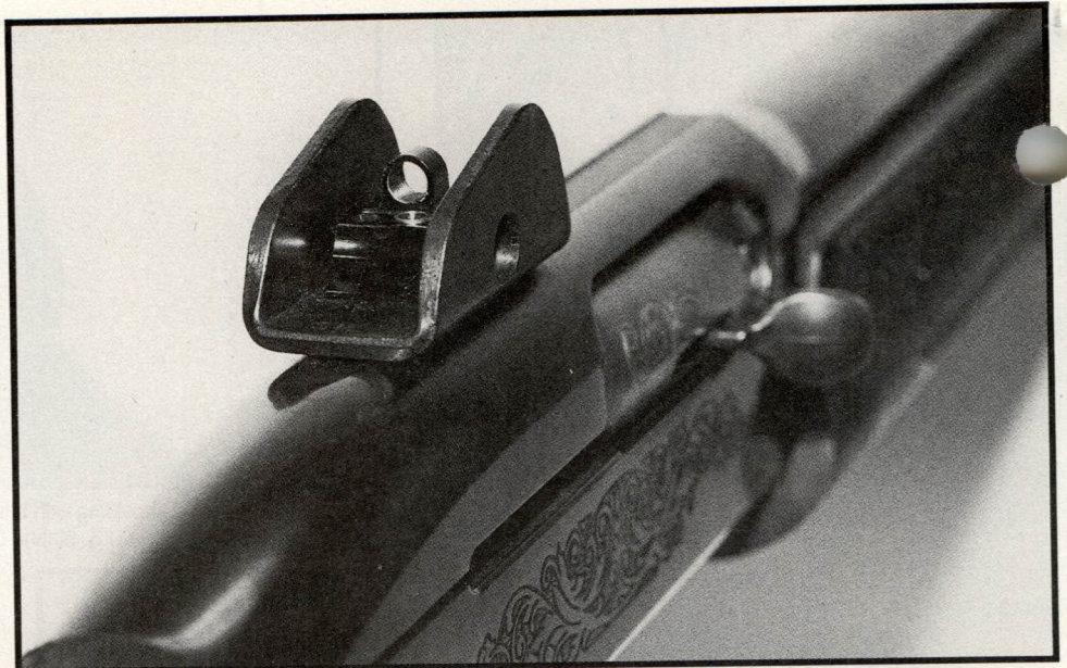
The Sage sight is basically an improvement of the Williams design. It's made of steel, while the Williams was made from an aluminum alloy.
